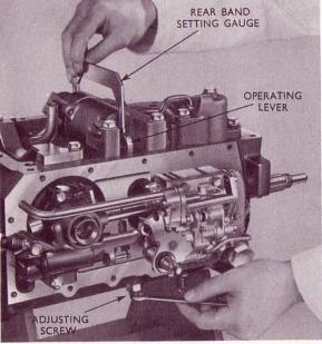
At left are the rear band adjusting tools the larger one is for the Shadow gearbox!
