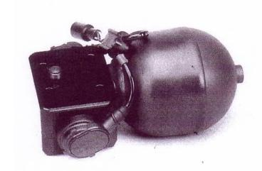
And at the top end of your rear dampers, a similar setup controls the in and out hydraulic traffic to the gas spheres.
