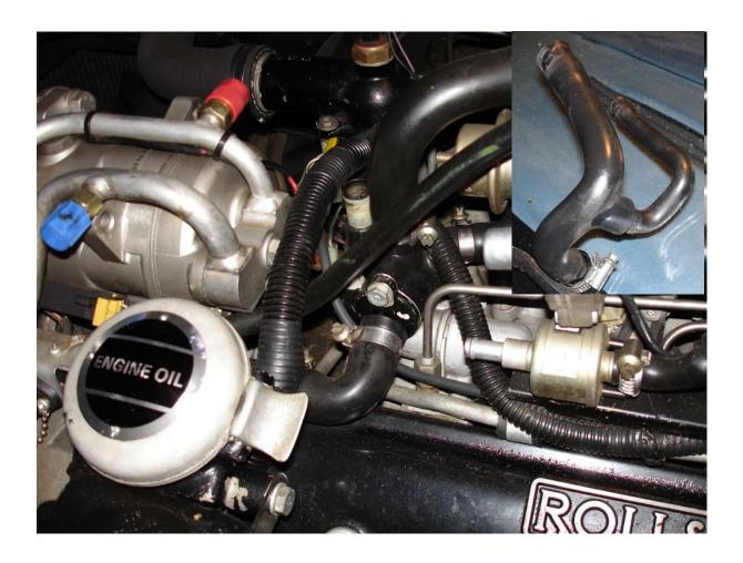
Well here we have removed the Pterodactyl's intestines (see inset) and the flame trap housing can now be clearly seen. Note the use on this model of the flexible plastic wiring sheaths. They are so practical, easily removed and replaced and don't unravel and collect dirt like the blasted insulation tape from previous years.
