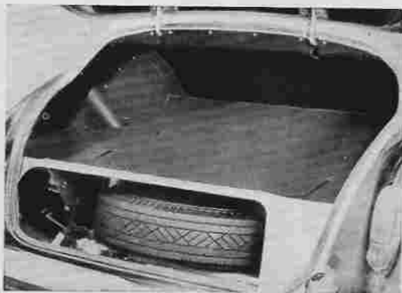
LONG and wide, with a virtually flat floor, the luggage boot of the new car has a separate compartment beneath it for spare wheel and battery.
