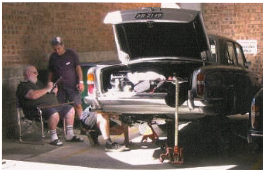
Doug Brown (seated) looks on as his 1974 Silver Shadow (SRH17894) receives new rear springs. Talking to Doug is believed to be Vegan Khacharourian.
