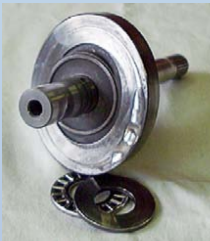
Disc and ball skidding, insufficient lubrication on the swashplate surface or foreign debris interrupting this process.
