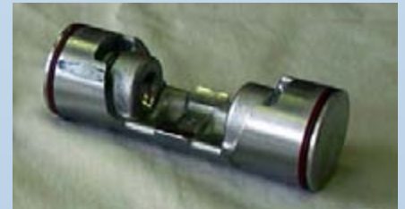
Piston damaged from 'grabbing' in the bore. Caused by insufficient 'barrier' lubrication between piston and bore.
