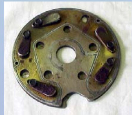
Corrosion caused by moisture contamination.
