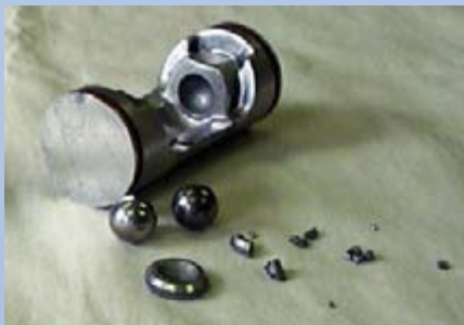
One disc fractured and matching ball damaged. The other disc almost fractured, skid marks on rear ball socket in piston out of shape.
