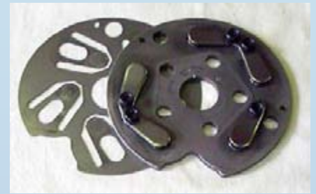
Valve plate discoloured from the black oil. Suction reed plate damaged from debris. Suction seats jammed with debris.
