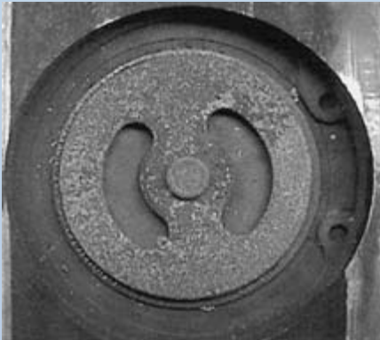
A flushing residue on the reed valve caused corrosion in this case.
