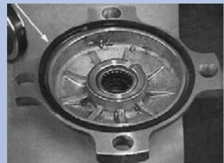
This seal swelled from a blend refrigerant. So it partly unseated and leaked.
