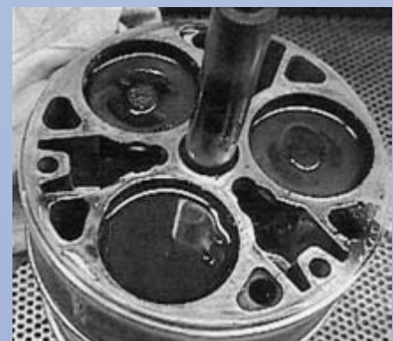
An unapproved flushing agent left residues that coated the cylinders, affecting performance.
