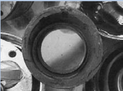
A flushing residue on the reed valve caused corrosion in this case.
