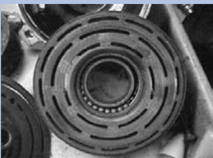
These clutch parts took a real beating, yet the cause was low refrigerant and frequent cycling, not the more commonly-thought-of high pressures and low voltage.
