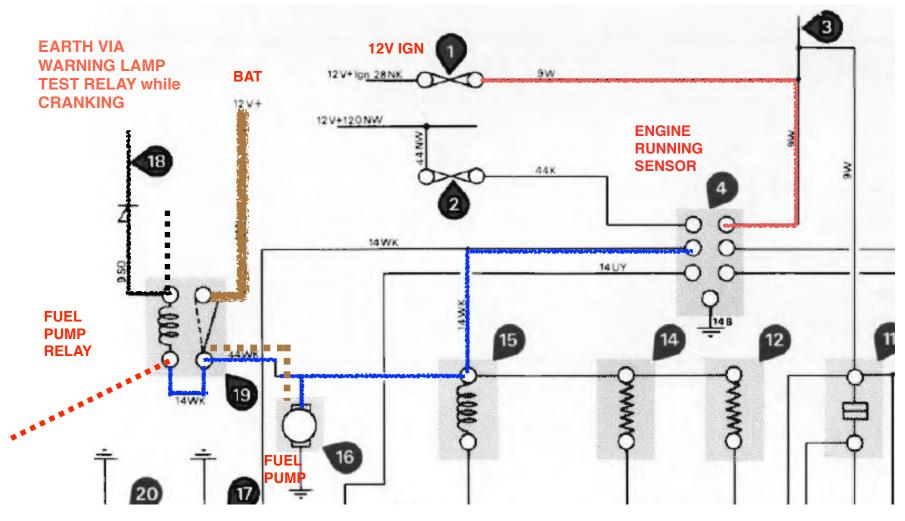
IGN ON = red circuit is powered, ERS energized
