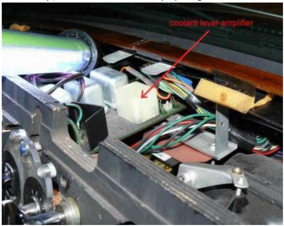
On the same board as those relays will be a whitish plastic cube, usually with its label intact, that reads: "UD 14927 Coolant Level." Carefully remove it from the relay board. After it is off the relay board, gently and carefully pry the circuit board out of the base of the cover. When that's done you should see something exactly like or very similar to this:
