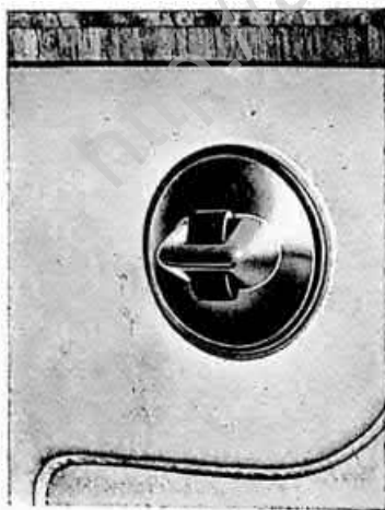
Fig 69 PASSENGER'S SWITCH FOR ELECTRICALLY OPERATED WINDOW
