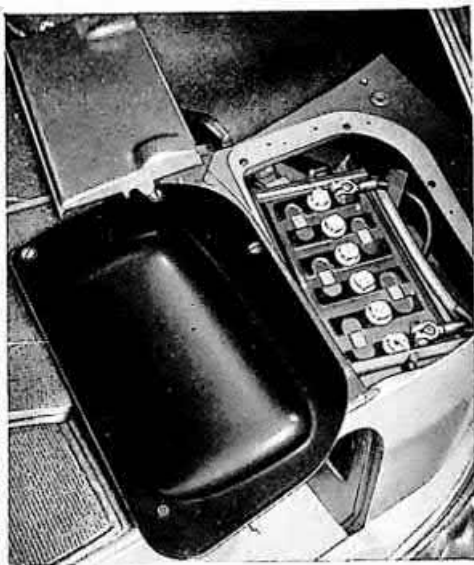
Fig 46 ACCESS TO THE BATTERY
