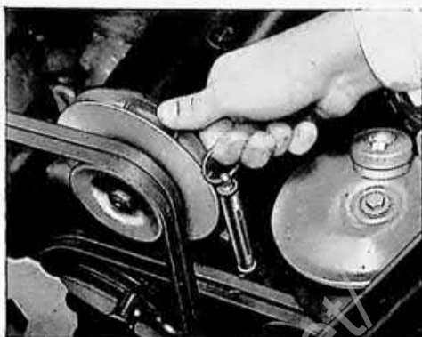
Fig 39 CHECKING TENSION OF STEERING PUMP BELTS
