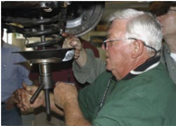
Our host compressing the front spring back into place.
