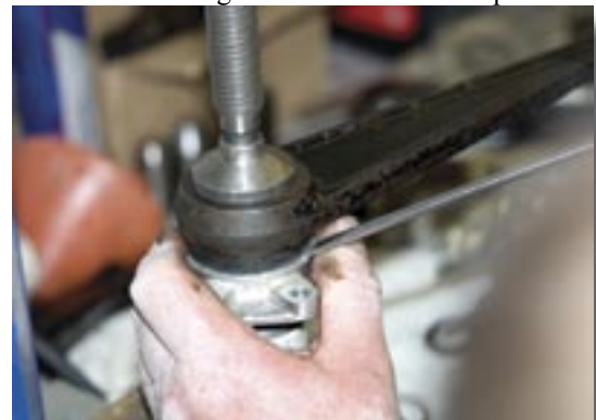
Guiding the rubber gasket into its housing.
