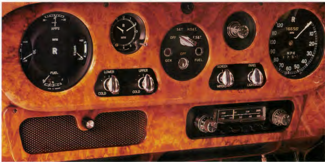
This 1962 Rolls-Royce instrument panel displays the 'R' motifs on the instruments. By this time, a rear speaker was fitted, and a balance control can be seen here above the speaker. The push-button Radiomobile is original.
