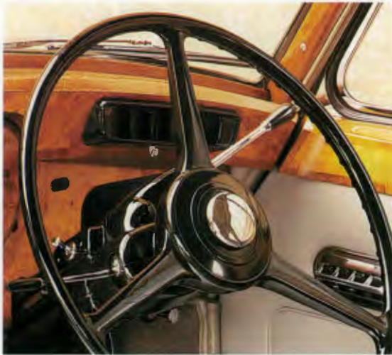
The steering column of this 1962 Silver Cloud carries the ride control switch and indicator headlamp flasher switch on its left side, while the automatic transmission quadrant is on the right. Visible on the door is the master switch for the electric windows.
