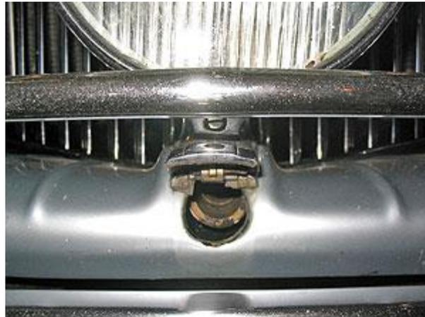
Fig E. shows the flap in the open position and also illustrates the modified starting handle guide with bronze bushing on R type B87UL.
