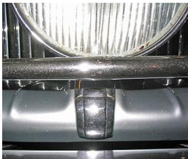
Fig D. Shows the flap in the closed position fitted to R type B87UL
