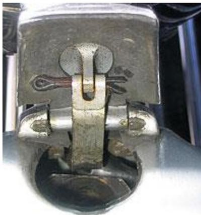
Fig G. shows the open flap, the image having been taken from slightly below the level of the flap. Also shown is the sheathed electrical harness to the centre driving lamp and the cut off top section of the modified starting handle guide together with the flap pin retention method.
