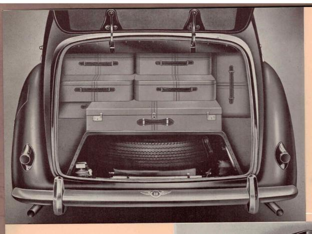
The extra large boot on the Bentley Saloon has a capacity of 17 cubic feet, sufficient space for a set of seven suitcases which have been specially designed for the car. The separate compartment affords easy access to the spare wheel and tools.
